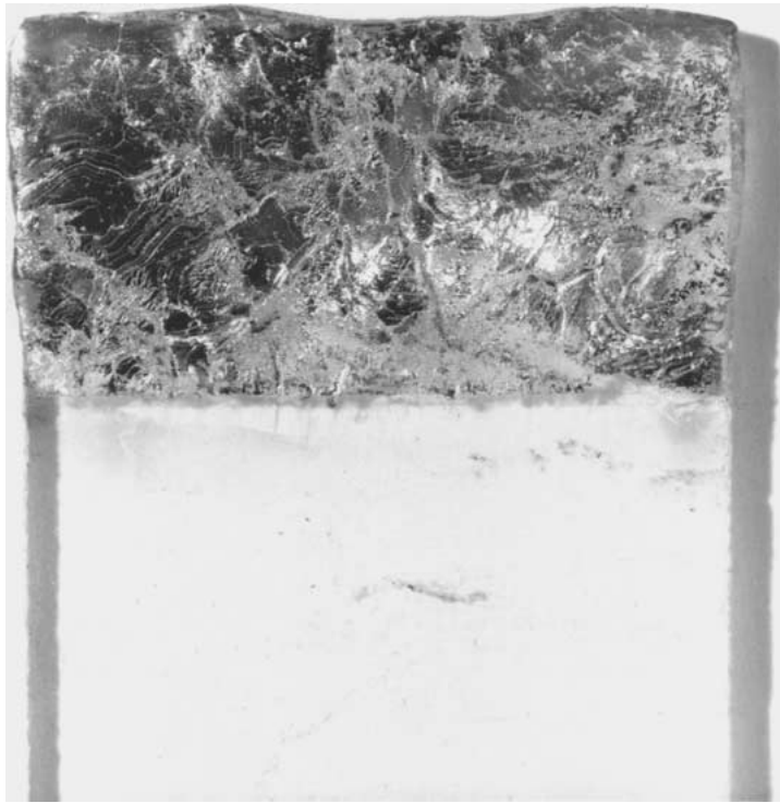
Figure 15 Gold sputter coated acrylic depicting crazing and material melt.
